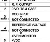
Note 1. If the specification does not specify parameters for either PIN3 or PIN4 then that respective PIN is NOT internally CONNECTED.
