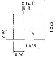
To ensure optimal oscillator performance, place a by-pass capacitor of 0.1uF as close to the part as possible between Vcc and GND PAD
