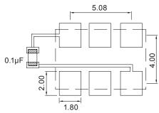
To ensure optimal oscillator performance, place a by-pass capacitor of  $0.1\mu F$  as close to the part as possible between Vdd and GND pads.
